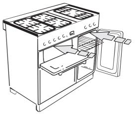
Open the grill door and right hand oven door so that you can get a good grip on the bottom of the fascia panel as you move the oven.
